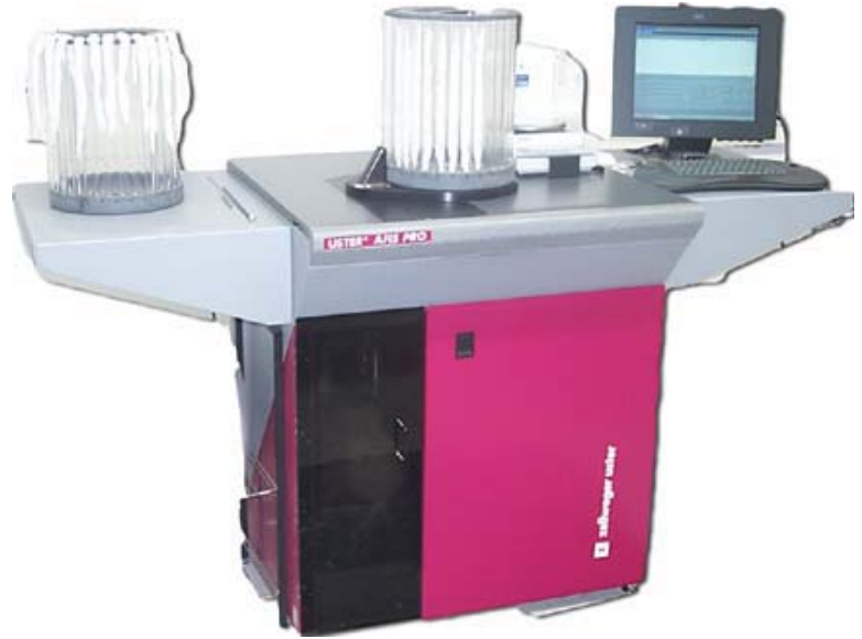
Exhibit 5: Advanced Fiber Information System (AFIS®) Source: International Textile Center
